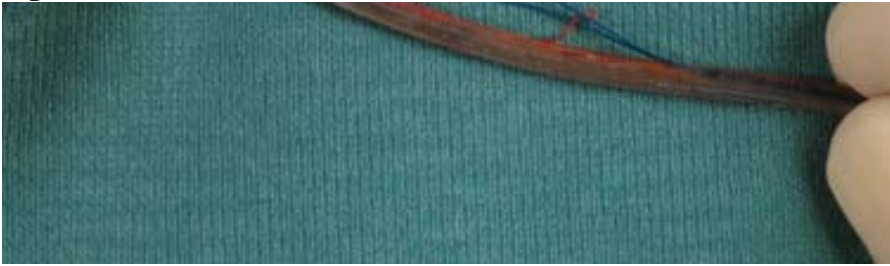
Figure A. Riata lead with externalization of conductor cables
